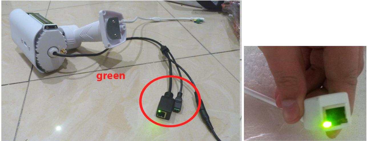
See below image, then you connect the RJ 45 cable to our IPC, ORANGE led should flash or keep lighted, below image shows the camera network cable is OK:
