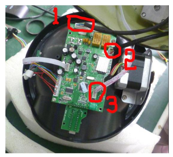
6. Now please cover the new housing to the PTZ, please be carefully, avoid to damage any cable. You must to connect the 3 cables of new housing to the decoder, please refer to my previous picture and the following picture.
