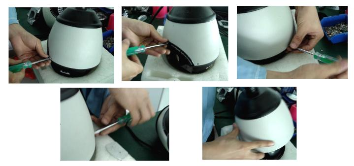
4. After you take off the PTZ's housing, you will see the decoder (main PCB board) on the top of ptz, but it is still connected to the housing via some wires, decoder is fixed by about 5 pcs screws.
