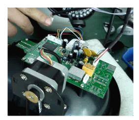
5. Now we need to take some wires on the decoder (PCB board) to change the housing. Please must to remember every positions of every wires, because you need to connect the decoder again later. Please take the 3 cables out that are as same as my following picture, when you change the new housing, you need to connect the 3 cables at new housing to these 3 positions, **please note**, **the cable NO.1**, **its position is the left socket near to the edge of decoder, but not the right socket**.
