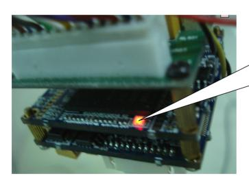
D1 light is blink means the IP module is connected to the computer, otherwise, means the connection is abnormal.
