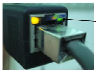
The green light should blink, otherwise, means the connection is abnormal, no signal.
