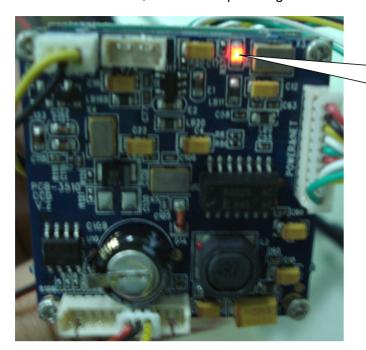
D5 light is on, means the IP module got power, ok.
