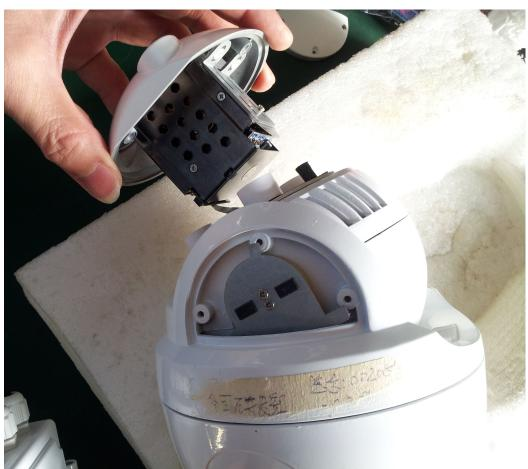
You can see the module is connected to the decoder via a flat cable, it is white, you need to open its lock, then you can take the cable off, please be lightly and carefully,
