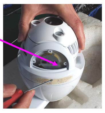
Now you can make the rest 2 screws to be tight, which are on left and right of the housing back. Finish replace zoom module of camera.
