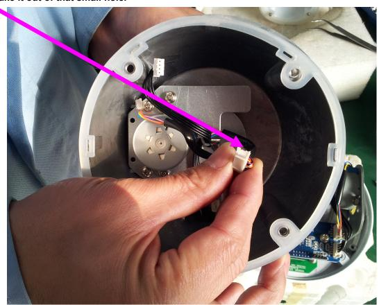
After you finish all works, please be carefully to fix all screws back to their original positions, and don't mix all screws together, for each part, put their screws separately, otherwise, some parts use different size of screws, and different style, when you found this lately, will waste your much time to do everything again.
