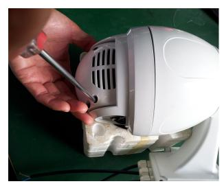
3. Now please turn the camera to the first position where you take 3 screws off, and you can see the parts like below picture, you need to use a screw driver to move a <a href="https://doi.org/10.1001/jibst.com/">https://doi.org/10.1001/jibst.com/</a> a screw driver to move a <a href="https://doi.org/">hidden part</a> out, <a href="https://doi.org/">just use the tool to feel it and lightly pull it out,
