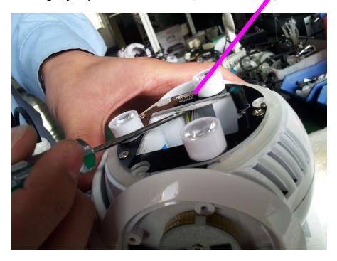
See the below 2 pictures, Please take the screws off, then you can take the module off, please note the side of module is different, this side you need to take off screws is without the cable connector, and remember its right position, otherwise, when you put it back later, will make big mistake.
