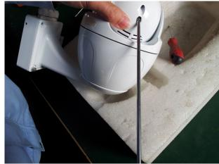
Then you need to push a small part into housing, it is at the position of ear which you opened, like below picture, this <a href="hidden part">hidden part</a> was pulled out when you did the 3<sup>rd</sup> step, just use the screw drive to push it lightly, then it will be hide again.
