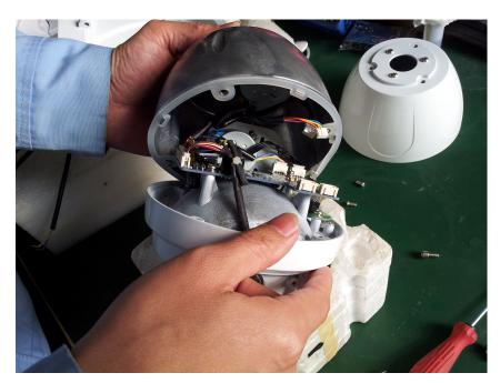
6. You need to pull 3 connectors out, the one behind Yellow IC and whit one on the picture on right:
