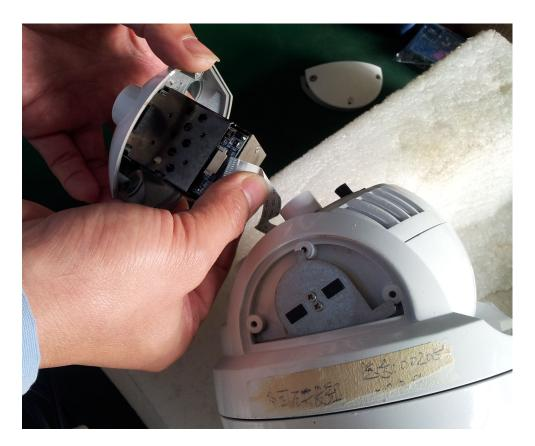
Now you can check if the connector is loosen, the position is under this part in my picture, if it is loosen, please make it tight, just push it into the socket, :
