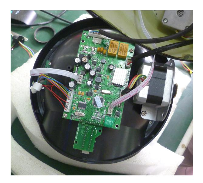
9. After you fix the new decoder, please cover the original PTZ housing, then put all screws of the housing and bracket to their original positions, make the housing and bracket to be stable, then you can test the camera again.
