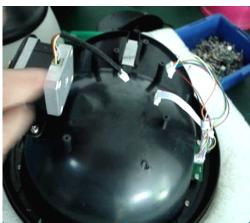
7. Now we can replace a new decoder to the PTZ, put the new decoder on the position of old decoder, and make it looks as same as before. Then use the screws to fix it on the PTZ's top. Please refer to my pictures, but not means you only need to fix 2 screws, you should fix all screws that you took off from the old decoder.
